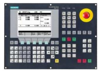
The SINUMERIK 802S base line is a CNC control that was developed for operation with up to 3 stepper drives and one analog spindle.
