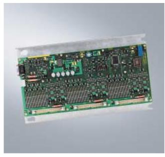
The I/O module PP 72/48 is connected to PROFIBUS DP and provides 72 digital inputs and 48 digital outputs. The 3 plug-in connectors for the inputs and outputs are 50-pole terminal posts for connecting ribbon cables. Application areas are with SINUMERIK 802D/802D base line.
