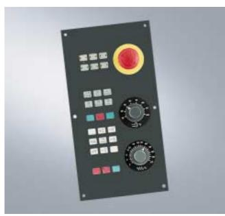
The MCP machine control panel for SINUMERIK 802D and SINUMERIK 802D base line provides an easy solution for turning and milling machines. All the keys required for operation are provided and can be directly connected to the PP 72/48 I/O module over a ribbon cable. The connections are made at the 24 V DC level and are therefore easy to implement.
