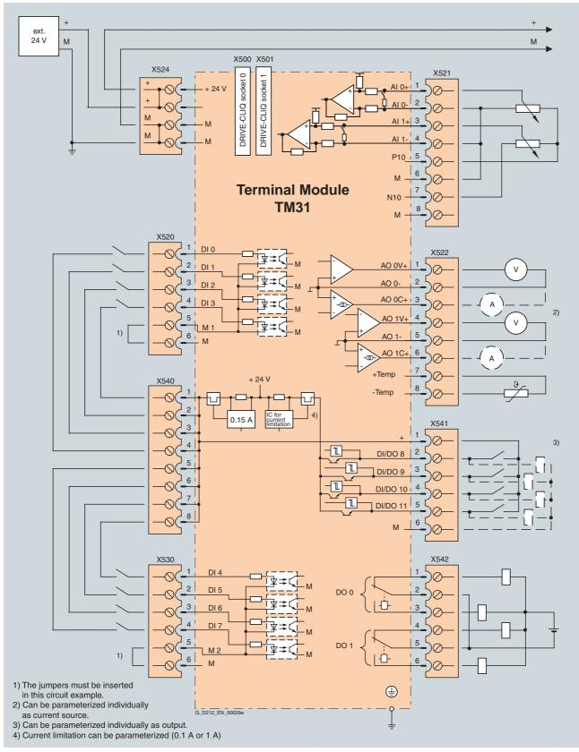
Connection example of a TM31 Terminal Module
