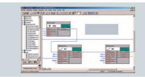
A sufficient number of free function blocks for various applications is included as standard. Optionally, the functional scope can be subsequently extended using free function blocks from Drive Control Chart (DCC). This allows the drive to be optimally adapted to the particular application – both technically and economically.
