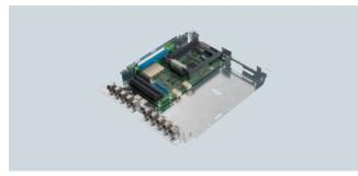
In addition to the connections and functions of the Standard CUD, the Advanced CUD has two DRIVE-CLiQ connections and one option slot. The use of an Advanced CUD also provides the opportunity of inserting an additional CUD (Standard or Advanced) to increase the computational performance and the number of terminals. This can be used, e.g. to implement additional technological functions.
