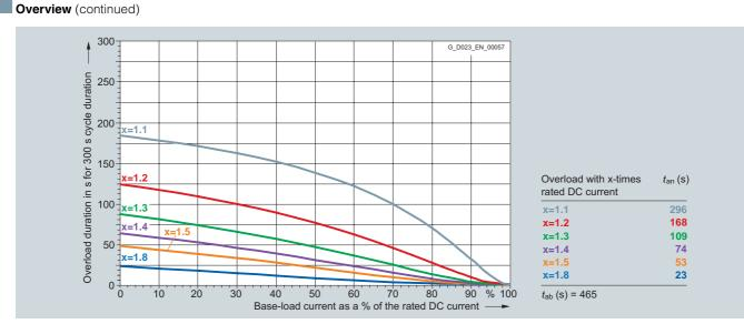
6RA8097-4KS22-0AA0 2 600 A/two-quadrant operation 690 V, 6RA8097-4KV62-0AA0 2 600 A/four-quadrant operation 690 V
