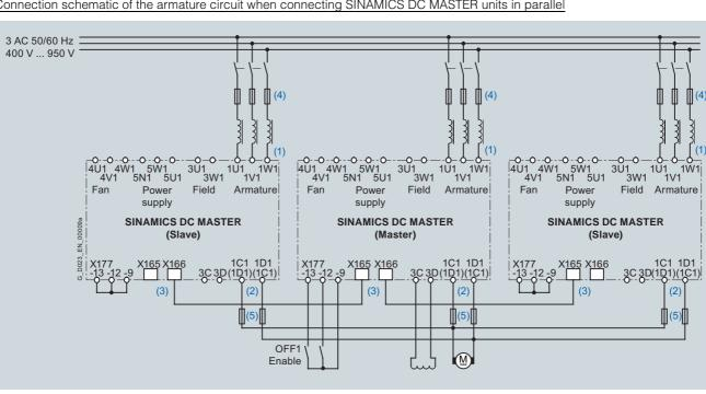
Connection schematic of the armature circuit when connecting SINAMICS DC MASTER units in parallel
