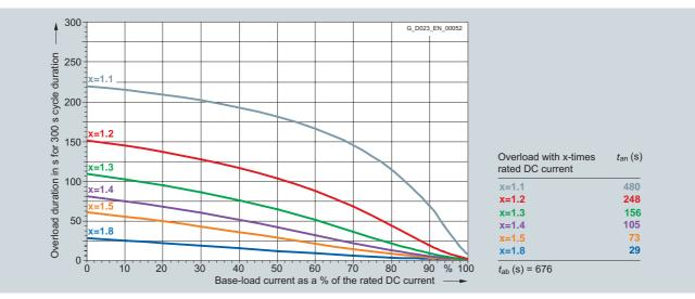
6RA8095-4KS22-0AA0 2 000 A/two-quadrant operation 690 V, 6RA8095-4KV62-0AA0 2 000 A/four-quadrant operation 690 V
