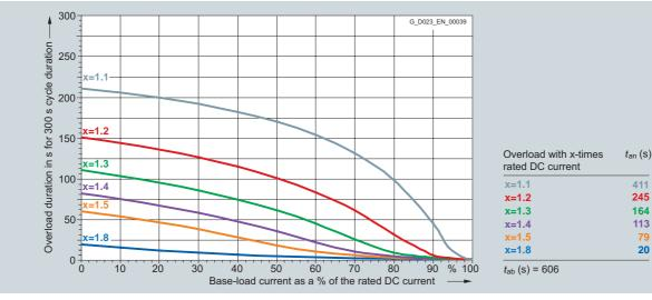
6RA8086-6KV62-0AA0 760 A/four-quadrant operation 690 V
