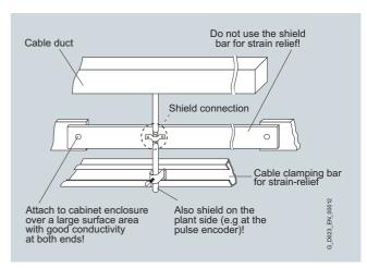
Shielding at the cable entry to the cabinet
