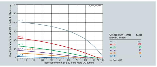
6RA8085-6DS22-0AA0 600 A/two-quadrant operation 400 V, 6RA8085-6FS22-0AA0 600 A/two-quadrant operation 480 V, 6RA8085-6GS22-0AA0 600 A/two-quadrant operation 575 V
