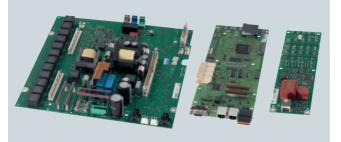
PCBs coated on both sides and nickel-plated copper busbars are two options to improve the reliability for increased degrees of pollution and climatic stressing – as well as for increased environmental stressing (e.g. for aggressive atmospheres).
