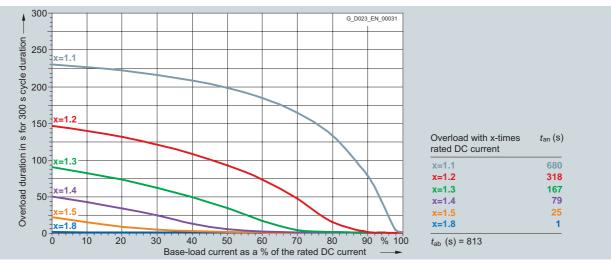
6RA8075-6DS22-0AA0 210 A/two-quadrant operation 400 V, 6RA8075-6DV62-0AA0 210 A/four-quadrant operation 400 V, 6RA8075-6FS22-0AA0 210 A/two-quadrant operation 480 V, 6RA8075-6FV62-0AA0 210 A/four-quadrant operation 480 V, 6RA8075-6GS22-0AA0 210 A/two-quadrant operation 575 V, 6RA8075-6GV62-0AA0 210 A/four-quadrant operation 575 V
