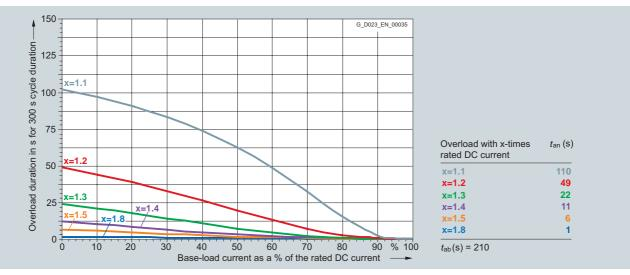
6RA8082-6FS22-0AA0 450 A/two-quadrant operation 480 V, 6RA8082-6FV62-0AA0 450 A/four-quadrant operation 480 V
