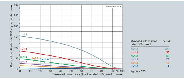
6RA8088-6LS22-0AA0 950 A/two-quadrant operation 830 V, 6RA8088-6LV62-0AA0 950 A/four-quadrant operation 830 V
