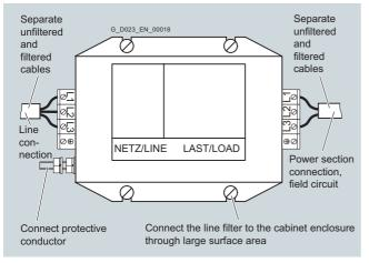
Radio interference suppression filter
