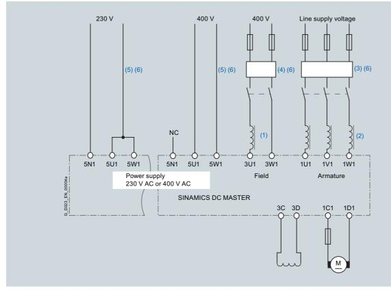
Arrangement of reactors and radio interference suppression filters
