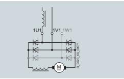
For units up to 125 A and up to 575 V AC, the full functionality is available even when supplied through just two conductors. This means, for example, that when retrofitting a converter with single-phase connection, it is not necessary to make any changes to the existing machine or plant – and the retrofitted drive system can be integrated into state-of-the-art communication concepts (TIA).
