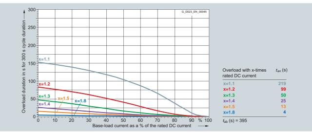
6RA8090-6KS22-0AA0 1 000 A/two-quadrant operation 690 V, 6RA8090-6KV62-0AA0 1 000 A/four-quadrant operation 690 V
