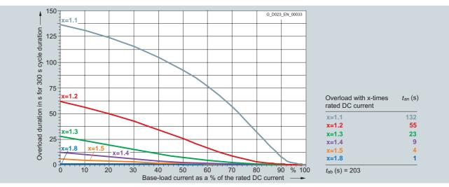
6RA8081-6DS22-0AA0 400 A/two-quadrant operation 400 V, 6RA8081-6GS22-0AA0 400 A/two-quadrant operation 575 V
