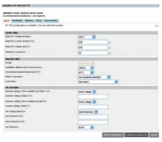
SIZER LD web is used when engineering SINAMICS DC MASTER. It provides supply when selecting and dimensioning the converter, associated options and accessories required for the particular application. SIZER LD web is implemented as web-based application (Internet): http://www.siemens.com/sizer-Id.
