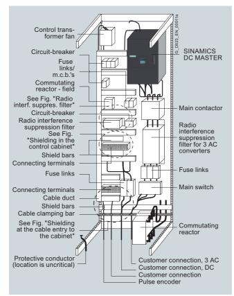
Example of a cabinet design with a SINAMICS DC MASTER of up to 850  $\mbox{A}$
