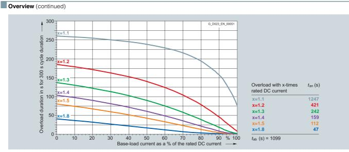
6RA8095-4GS22-0AA0 2 000 A/two-guadrant operation 575 V, 6RA8095-4GV62-0AA0 2 000 A/four-guadrant operation 575 V
