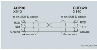
Assignment of the RS232 cable for connecting to an AC SINAMICS unit (not for SINAMICS DC MASTER!)
