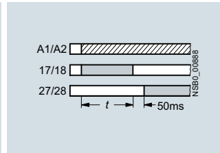
I 7PV1508-1B Fixed pulse after ON-delay
