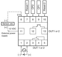
Note: Each output can be flexibly allocated to either stage 1 or 2 by setting in function selection mode.
