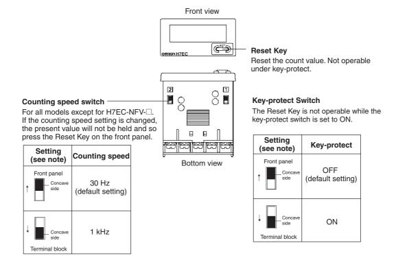
Note: Perform switch setting before mounting to a control panel.
