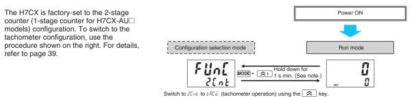
Note: The MODE key must be pressed before the <a>1</a> key.
