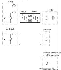
1. Contact Input (Input by a Relay or Switch Contact)
