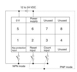
H7GP-T External power supply 12 VDC 50mA max. 100 to 240 VAC Ń Power Powe 0 V 12 VDC supply supply 7 5 6 8 2 3 1 4 Count input Reset Key protectio Unused input input Ś NPN mode PNP mode
