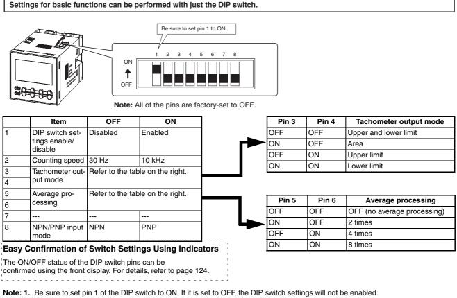
2. Changes to DIP switch settings are enabled when the power is turned ON.
