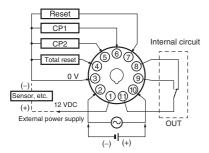
Note: Do not connect unused terminals as relay terminals.
