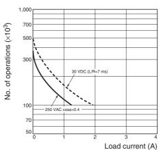
Reference: <u>A current of 0.15 A max. can be switched at 125 VDC (cos $\phi$ =1)</u> and current of 0.1 A max. can be switched if L/R=7 ms. In both cases, a life of 100,000 operations can be expected. The minimum applicable load is 10 mA at 5 VDC (failure level: P).
