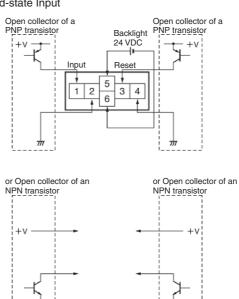
Note: 1. Terminals 2 and 4 (input circuit and reset circuit) are functionally isolated.
