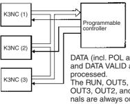
DATA (incl. POL and OVER) and DATA VALID are wired-OR processed. The RUN, OUT5, OUT4, OUT3, OUT2, and OUT1 signals are always output regardless of the status of the REQ signal. Do not OR-wire these signals.
