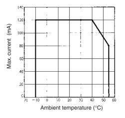
Note: The derating curve shown is for standard installation. The derating curve depends on the mounting direction.
