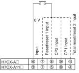
Operates when the contact turns ON.
