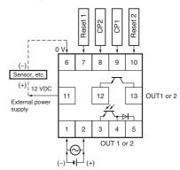
Note: Each output can be flexibly allocated to either stage 1 or 2 in function selection mode.
