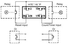
When the H7EC-NP is used, relay chattering may be counted. Use the H7EC-NLP, one of the low-speed input models.
