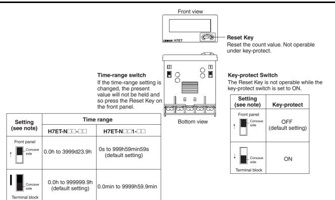
Note: Perform switch setting before mounting to a control panel.
