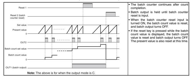
Note: 1. The batch count value is held at 0 during batch counter reset input.
