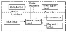
Note: All models except for H7CX-DD (models with 12 to 24-VDC power supplies) have basic insulation.
