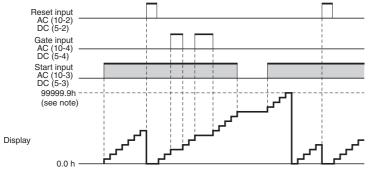
Note: 1. Display values are shown for full scale set to 99999.9 h. 2. Gate input is available only when H7HP-A settings are made.
