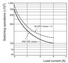
Reference: A maximum current of 0.15 A can be switched at 125 VDC  $(\cos\phi = 1)$  and a maximum current of 0.1 A can be switched if L/R is 7 ms. In both cases, <u>a life of 100,000 operations can be expected.</u> The minimum applicable load is 10 mA at 5 VDC (failure level: P).
