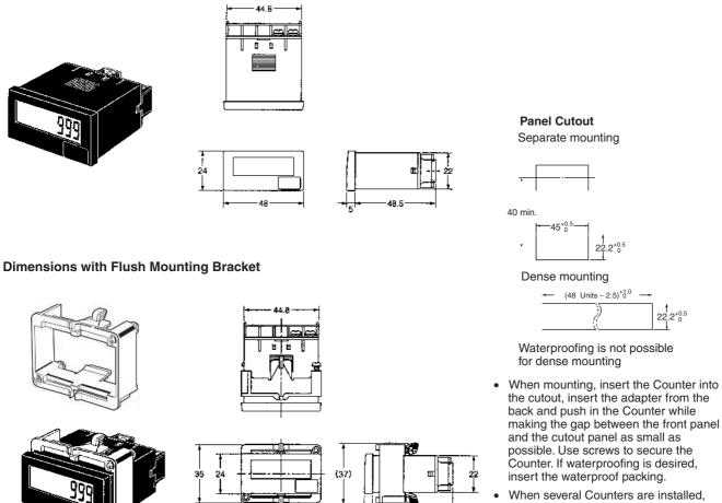
insert the waterproof packing. When several Counters are installed, ensure that the ambient temperature will not exceed specifications.
