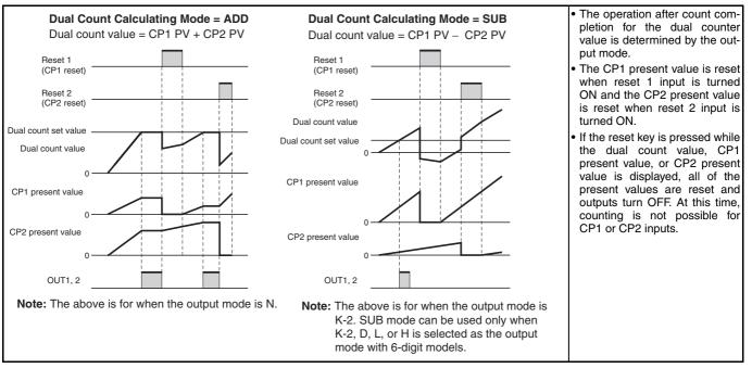
Note: 1. Counting is not possible for CP1 during reset 1 input. CP2 will not be affected. The dual count value will be calculated based on a CP1 present value of 0.
