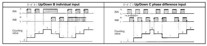
Note: 1. "B" must be larger than half the minimum signal width. If it is smaller, an error of  $\pm 1$  count may occur.
