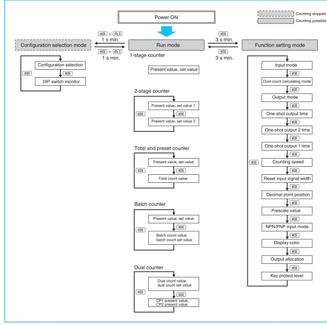
Note: 1. Perform settings using the a and b keys (a key only with 6-digit models).
