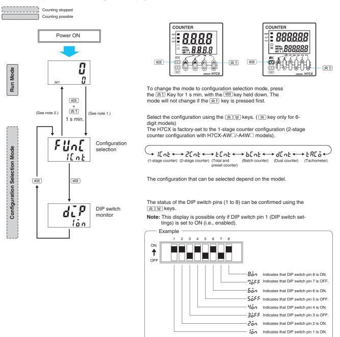
Note: 1. When the mode is changed to configuration selection mode, the present value is reset, outputs turns OFF, and counting (measuring) stops.
