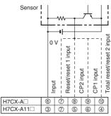
Operates when the transistor turns ON.
