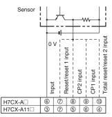
Operates when the transistor turns OFF.
