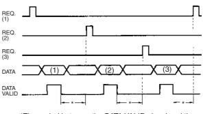
\*The period between the DATA VALID signal and the REQ signal should be no less than 20 ms max.
