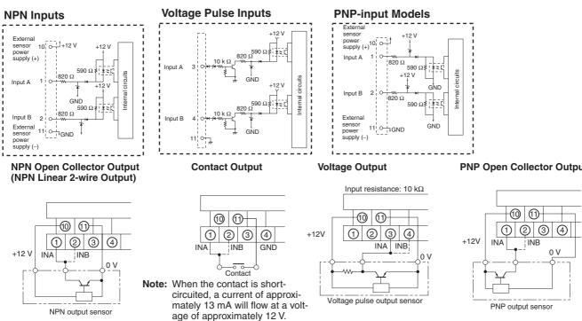
Note: Connect the + side of the NPN linear 2-wire input to terminal 1 and the - side to terminal 11.
