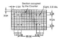
Note: Processing dimensions are for 28-pin IC socket.
