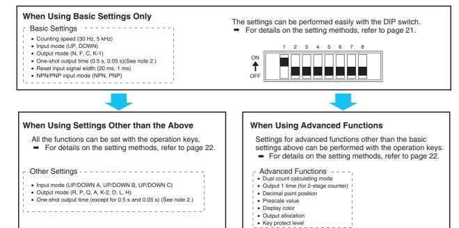
Note: 1. At the time of delivery, the H7CX is set to the 1-stage counter (2-stage counter for H7CX-AW□/-A4W□ models) configuration. 2. Set to output 2 time when using as a 2-stage counter or batch counter.
