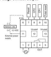
H7CX-AS/-A4S 1-stage Transistor Output
