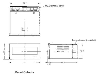
Panel cutouts are as shown below (according to DIN43700).
