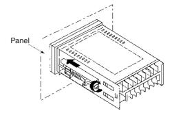
Attach the mounting bracket on the left and right sides of the Counting Meter as shown in the illustration above and gradually tighten each screw evenly in turn by considering the balance of the tightening force until the ratchets start slipping without being further tightened.
