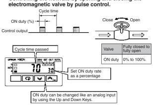
Refer to *Input/Output Mode Settings* on page 82 for information on ON/OFF-duty adjustable flicker mode operation.
