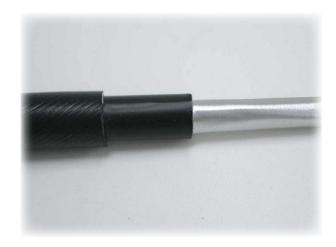
This design combining aluminium tape and HDPE sheath with a covering of polyamide PA (Nylon), represents an excellent barrier against penetrating chemicals and can be used as an alternative to lead sheath.
