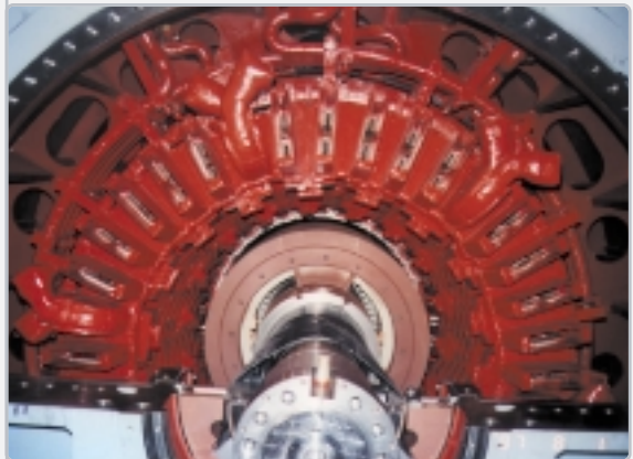
150MVA, 3,600RPM, 13.8kV, Open Air Cooled
