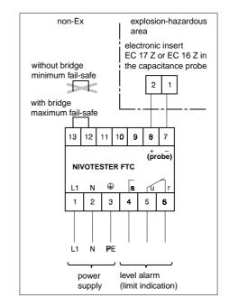
Electrical connections to the probe, power. signalling and control instruments
