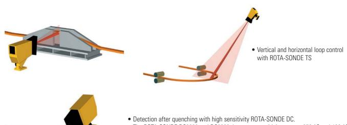
The ROTA-SONDE DC3000 and DC6000, have two sensitivity ranges, 250 °C and 400 °C. The range can be remotely selected. This feature makes the ROTA-SONDE DC well adapted for the application where the change in the process or the type of material results in a significant variation of the temperature of the product or a variation of its emissivity factor.
