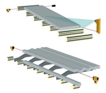
• Slab length measurement with TRILAS-TL and laser barrier V5
