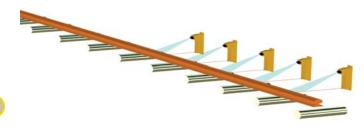
• Inline straightness measurement with laser sensor TRILAS-TL
