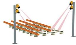
Detection of bloom or billet for cut to length with ROTA-SONDE DC. The scanning principle of the ROTA-SONDE enables a very accurate detection even with the sensor placed several meters away from the product
