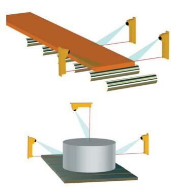
• Width measurement after reheat furnace or roughing mill with laser measurement sensor TRILAS-TL
