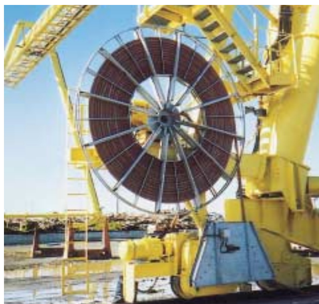
A Cavotec Specimas cable reel working at \pm 200 m/min on a P&H log-handling crane for Federal Paper Board, in Augusta USA.
