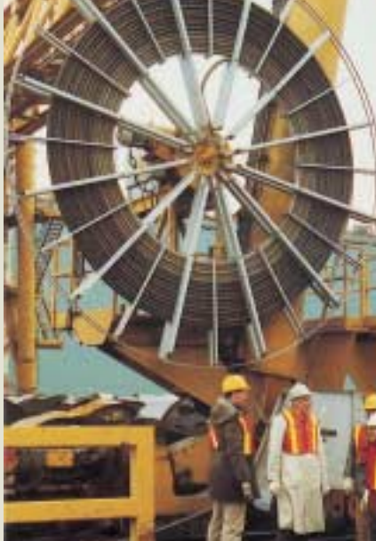
A large, high speed Cavotec Specimas cable reel mounted on a coil handler running at 180 m/minute.
