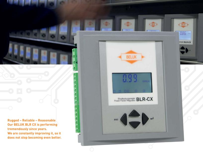
The BLR CX Series is a user-friendly "plug'n'play" device, that is designed to start regulating Cos Phi with a minimum of user interaction. Should further settings in the areas of measuring, regulating or alarms become necessary, the BLR CX offers a password protected expert-setup. All adjustments are possible during operation. Malfunctions of the compensation unit will be highlighted in the display and optionally trigger an isolated alarm relay.
