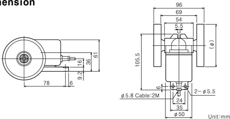
※A diameter( $\phi$ ) of wheel can be changed by application.
