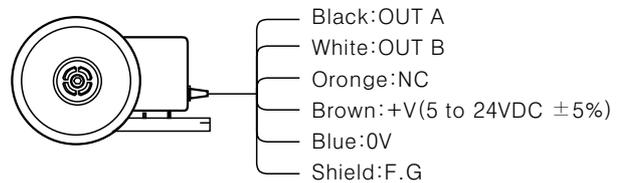
※Non-using wires must be insulated.
