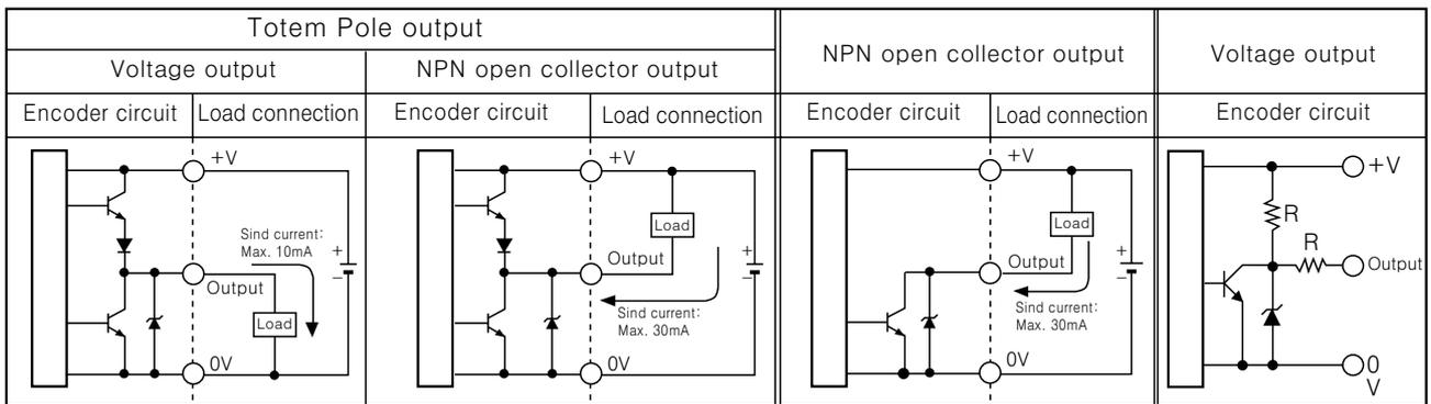
※The output circuit of A, B phase is the same.
