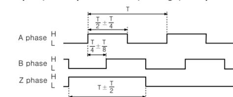
※The output waveform of E40 Series, NPN open collector is opposed to above waveform.
