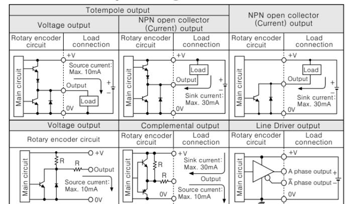
※All output circuit is the same A, B, Z phase(Line driver output is A, Ā, B, B̄, Z, Z̄)
