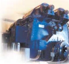
Low speed motors for cycloconverter applications. These low speed, high power machines are used on LCI systems for special applications. These motors are designed to withstand the fatigue stresses caused by extreme variable load and speed variations/reversals to ensure high reliability performance to the end user. (photo at top)
